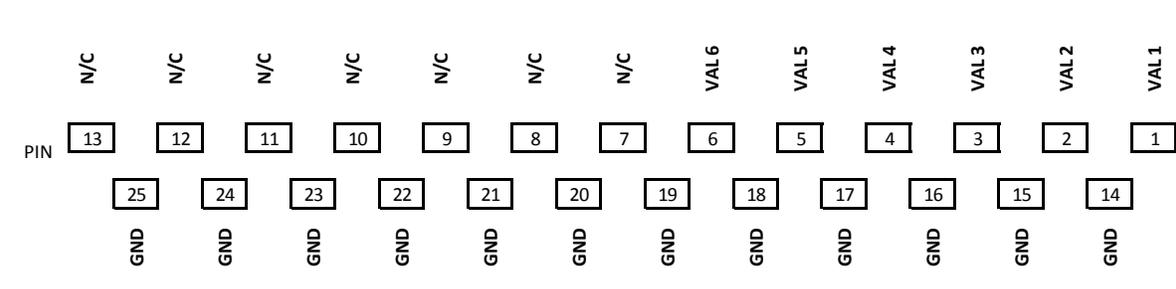
Figure 9 – DB25 Solenoid Output Connector Pin-Out
