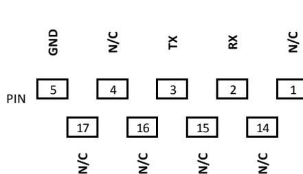
Figure 10 - DE9 Serial Communications Connector Pin-Out
